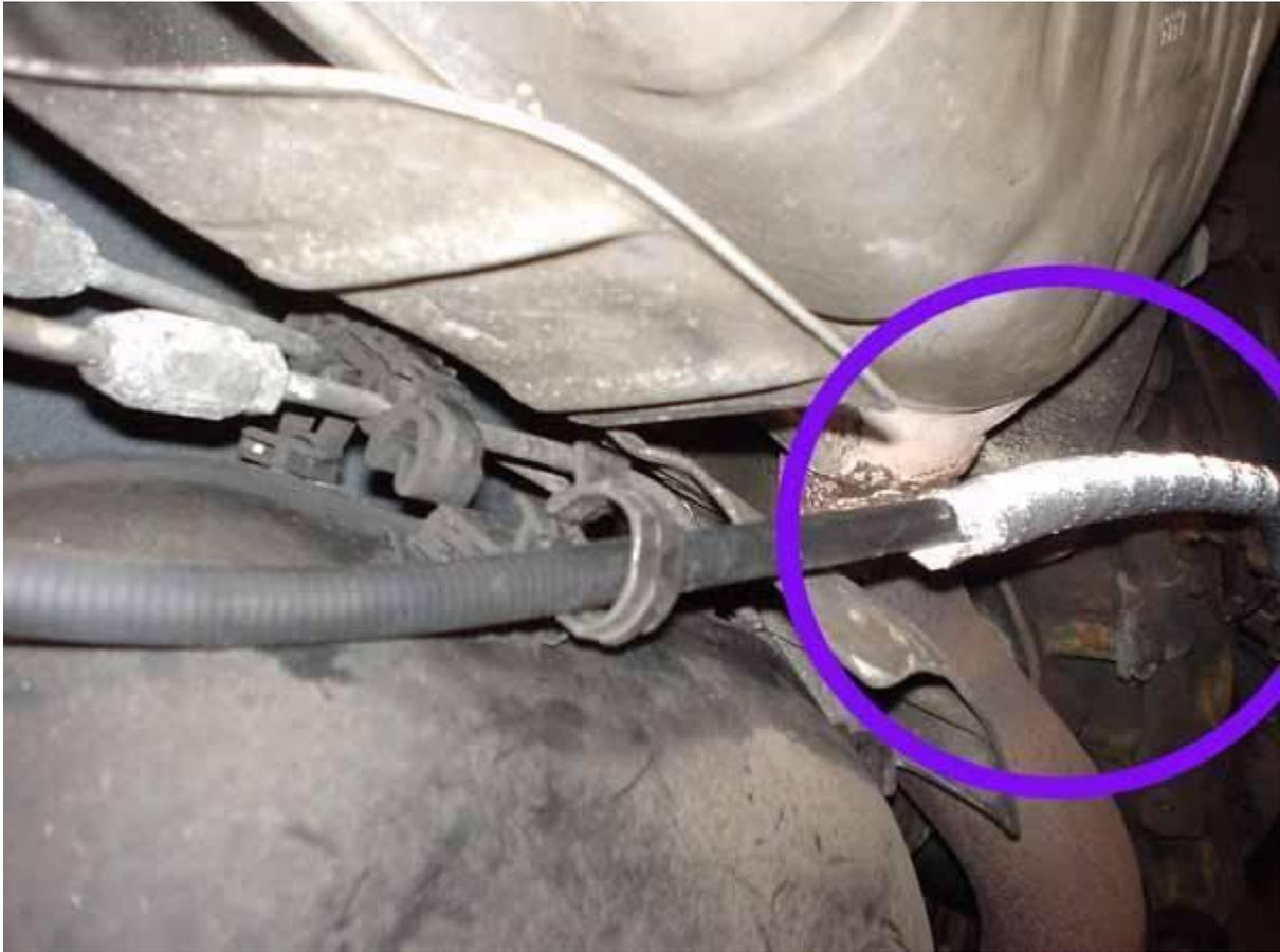
On the exhaust side you'll find this aluminium sheath which protects the exposed section from heat damage.
