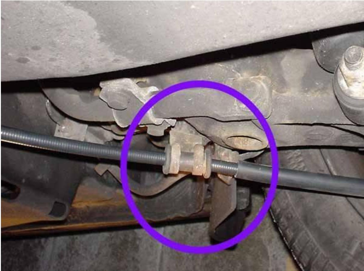
Also on both sides of the car you'll find these supports. The cable sits in them but you'll need to unbolt the 13mm bolt that holds the supports' bracket on to make room to slip the cable out.
