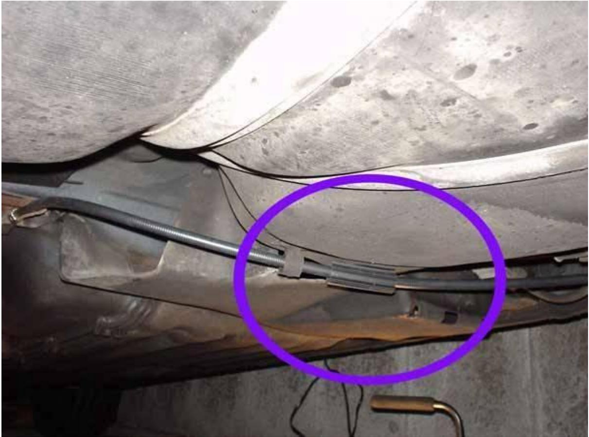
On the side of the car away from the exhaust you'll find this small free moving plastic widget. This stops the cable chafing on the tank.
