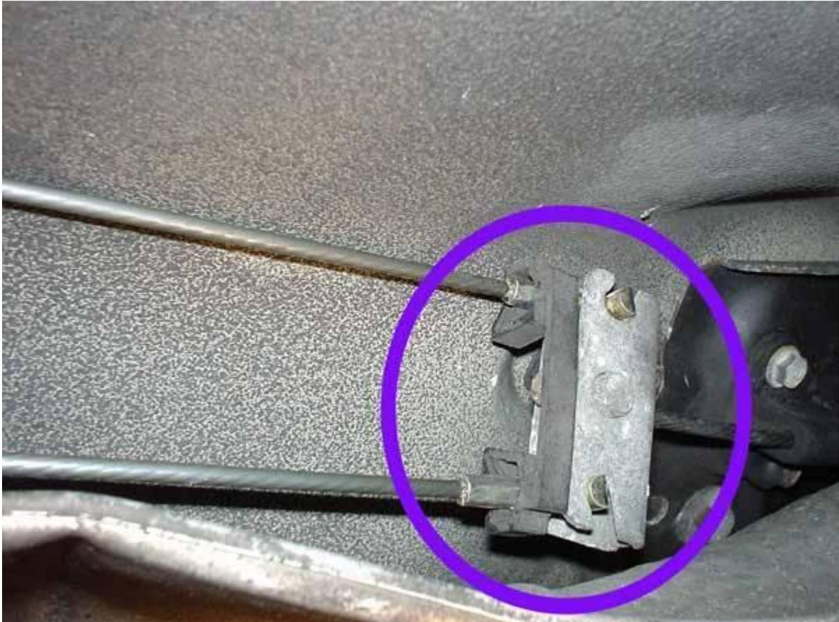
Now release the ends of the cables from the tie bar. This is in the middle of the car underneath and is easily accessible. Just remove the plastic clip and turn the cable ends out of the slots.
