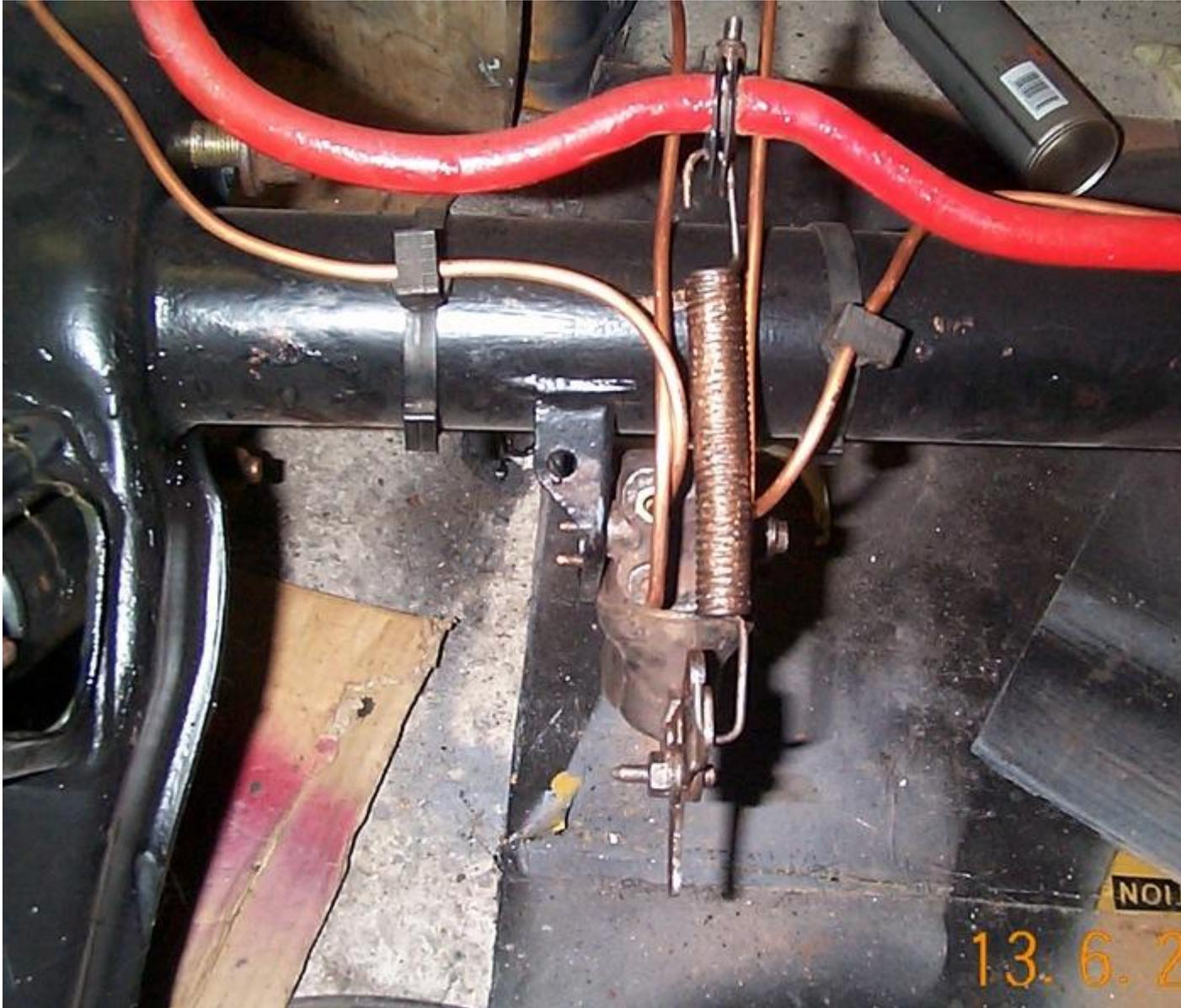
The idea is that under hard braking as the nose of the car dips, and the rear rises, the valve reduces pressure to the rear callipers to prevent the brakes from locking. So if the valve has seized in this position foot brake efficiency at the MOT will be poor. It is worth checking the condition of the rubber boot occasionally and giving the area behind the boot a good spray of copper grease every year or so..
