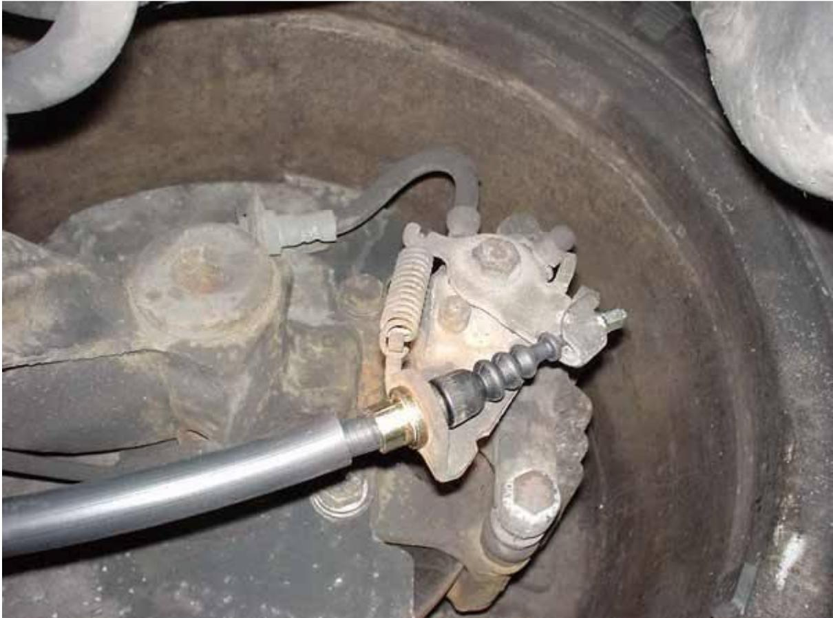
Finally, BEFORE connecting the new cables to the calliper slacken off handbrake cable, pump brake pedal 10 times with car level and all four wheels on ground.
